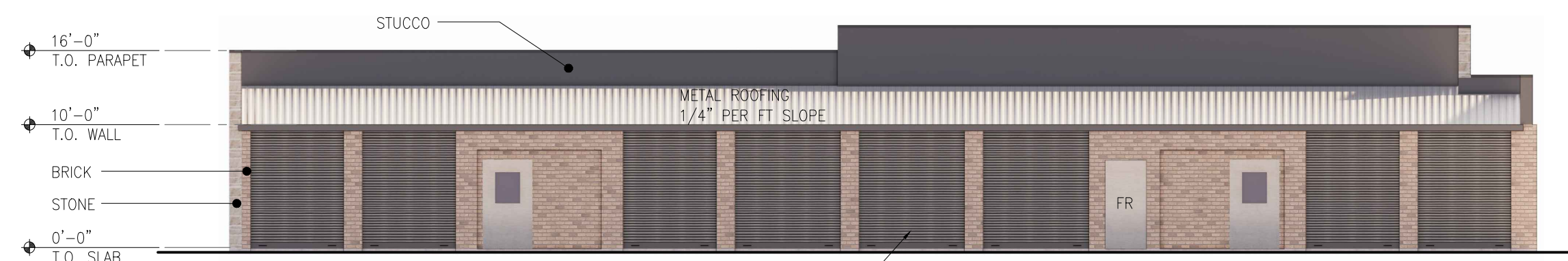
BLDG D NORTH ELEVATION SCALE: 3/32" = 1'-0"
